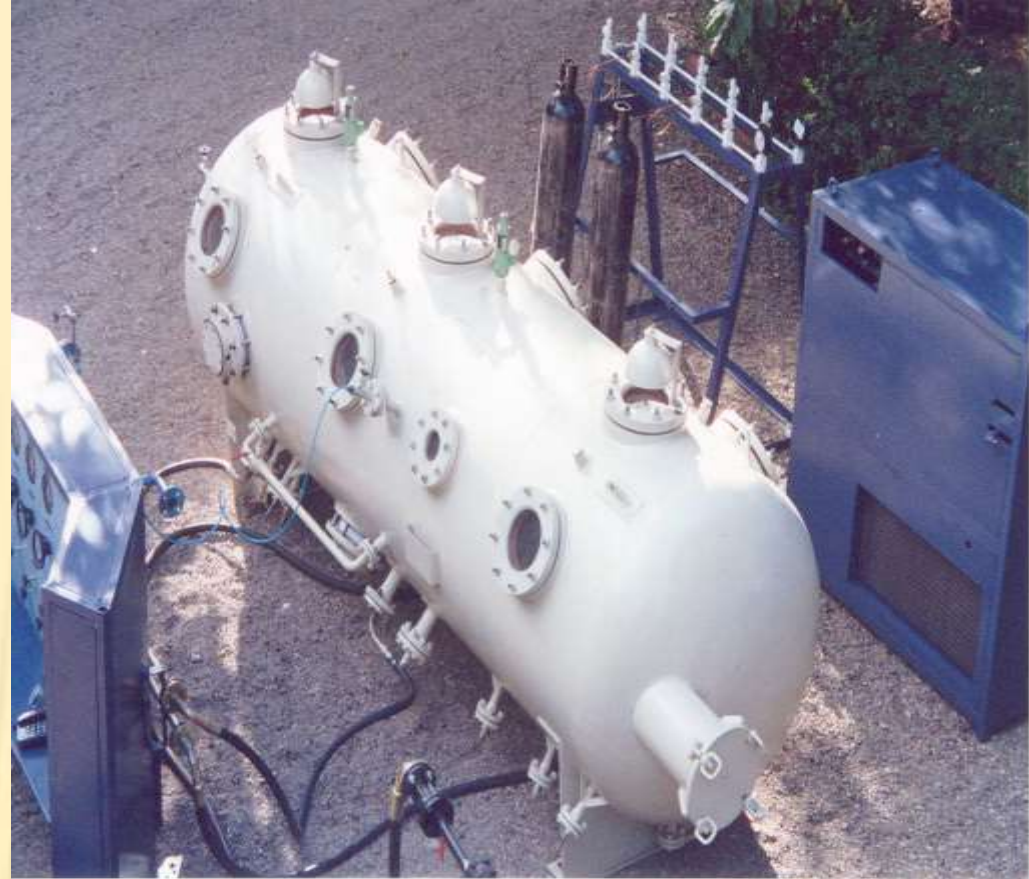
Monoplace Chamber with Air Lock Chamber at North Sikkim
